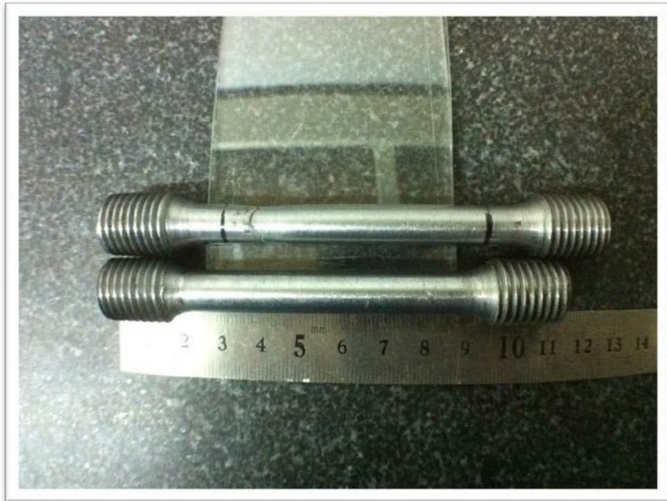
Fig 9: General plan of specimen after destructive test. Evident the difference between used one and unused.
