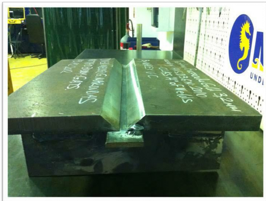
Fig 2: Test sample before welding, showing prep detail.
