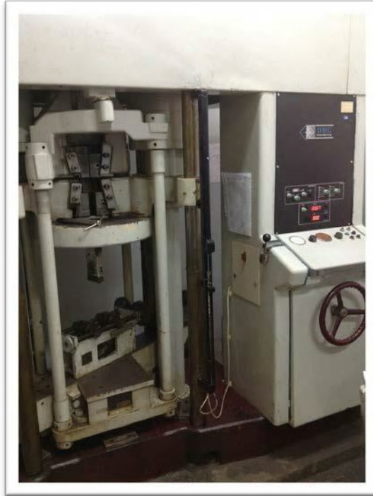
Fig 7: G.A.T.S. Ltd Laboratories. Tensile Machine, model DMG-T4284.
