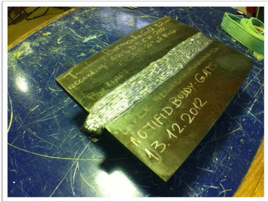
Fig 3: Test Piece as welded, looking side "A" to "B".
