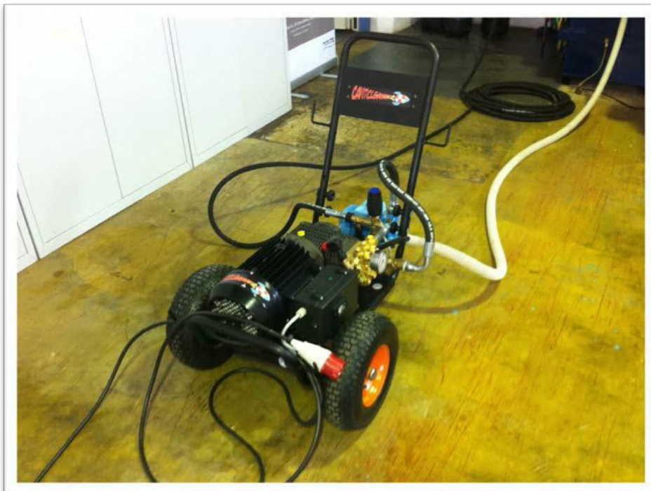
Fig 6: The cleaning system we used during the trial, called “ Cavicleaner ”.
